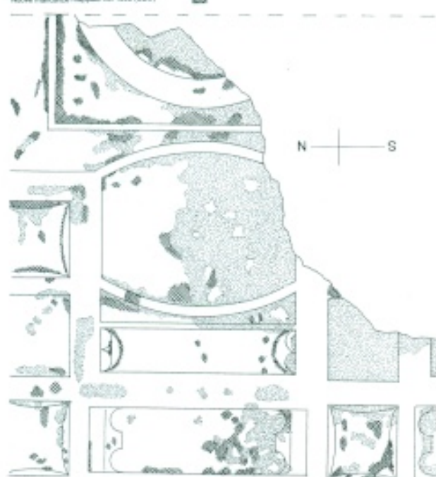
[1] Domus Aurea. A map of part of the Vault, the light grey showing losses in 1983 and the dark grey further losses occurring in just the 15 years to the treatment in 1998-99.
